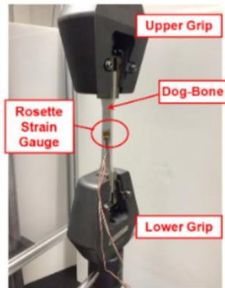
**Figure 2.** This figure depicts the lab setup for the tensile test using a recycled aluminum brass sample, Instron 8516 with an 80 [kN] load cell, and  $45^\circ$  strain rosette.
