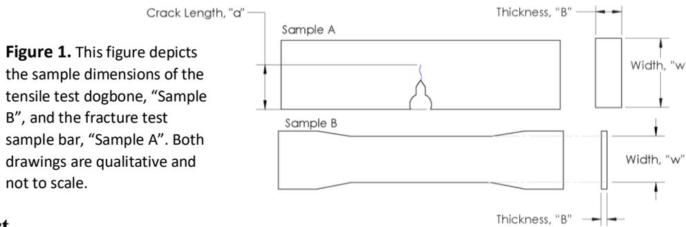
**Figure 1.** This figure depicts the sample dimensions of the tensile test dogbone, “Sample B”, and the fracture test sample bar, “Sample A”. Both drawings are qualitative and not to scale.
