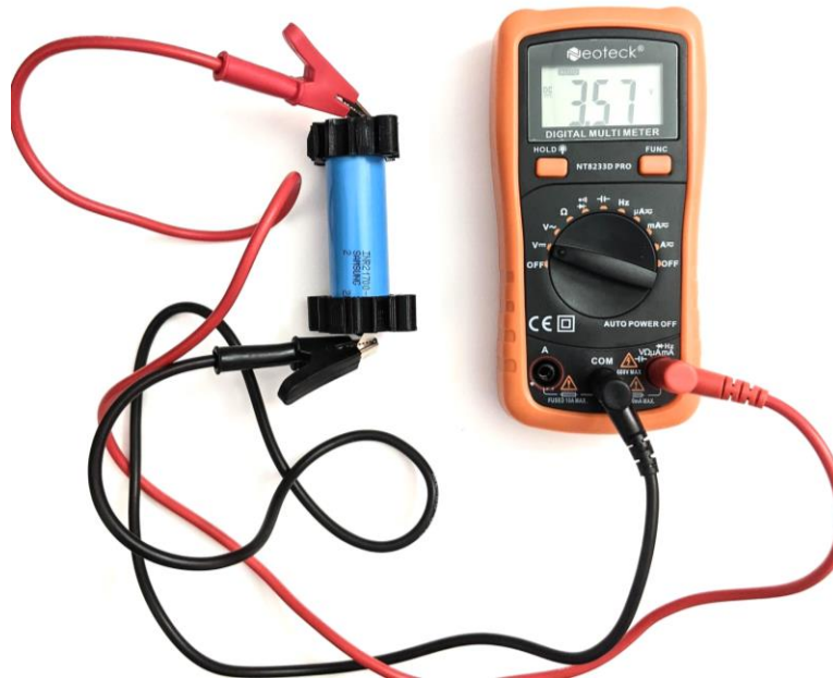
Figure 18. A Samsung INR21700-50E lithium-ion battery cell in a custom prototyping housing connected to a voltmeter to test the connection of the battery to the nickel plated copper busbar via press fit housing to battery interface.
