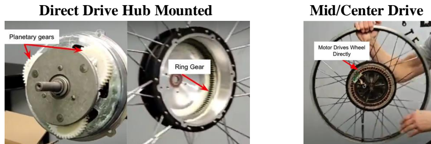
Figure 2. This figure shows images of the different types of motors used in drive systems of E-bikes.
